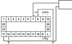
Connection with external 24VDC supply:
